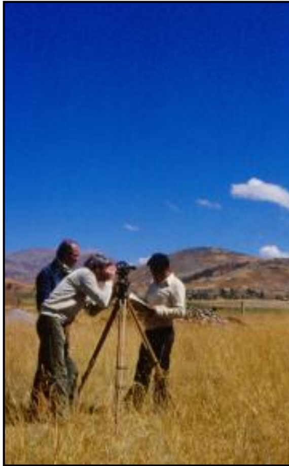
Fig. 9: Surveying the site to select an area without obstructions to install the pyranometer.
